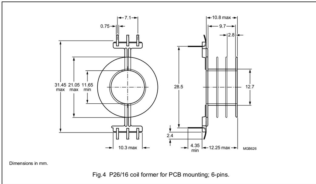
Winding data and area product for 6-pins P26/16 coil former for PCB mounting
